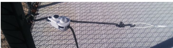
Figure 2: Large Rope Lock installed on the adjustable pole side and hooked onto game net cable loop with about 12" of rope between the rope lock and hook.
